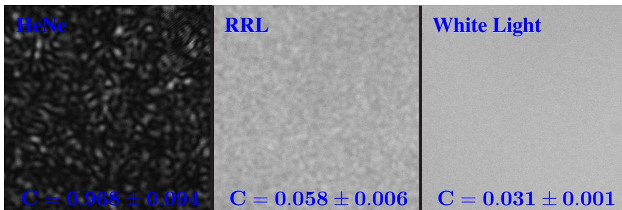
Figure 3. Speckle contrast of random Raman lasing. The speckle contrast measurements for a helium-neon laser and a halogen white light are shown for comparison and to illustrate the dynamic range of the measurement technique. This predicts 300 independent lasing modes present in the random Raman laser emission.
