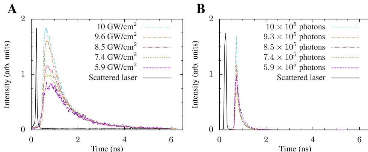
Figure 1. The temporal profile of the random Raman laser emission versus pump energy. (A) is the experimental data and (B) is the results of non-linear Monte Carlo simulations. The elastically scattered pump is shown for reference. Each trace has been normalized so that the exponential tails overlap by fitting an exponential decay and dividing each trace by the normalization coefficient. The exponential decay appears independent of pump power.
